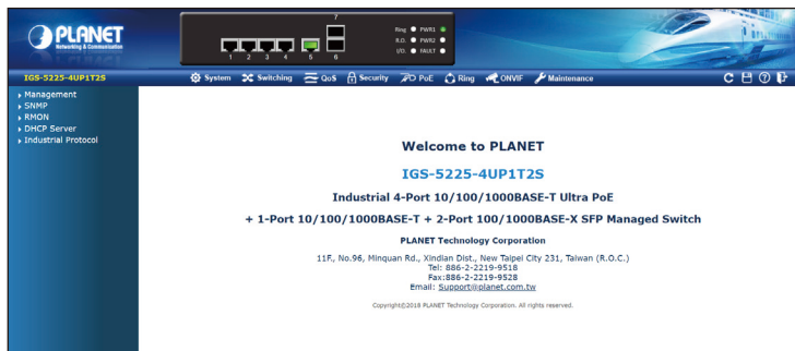
Figure 5-3: Web Main Screen of Industrial Managed Switch
