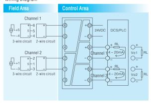
Note: above is wiring diagram of 2-wire circuit. Series with 1 in 2 out only connect input terminal with Channel 1, with 1 in 1 out connect input terminal and output terminal with Channel 1.
