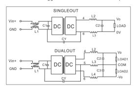
L2/L3/L4, C2/C3: forming the LC filter network to reduce the input ripple (the parameters of the devices are based on the ripple, but they can not exceed the maximum capacitive load)
