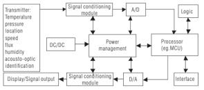
Typical application structure of signal conditioning module
