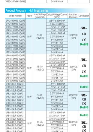
Note: 1. Chassis mounting and DIN-Rail mounting are available and please contact our sales department or refer to datasheet for details. Series have input reverse voltage protection
