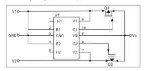
As the redundant design of diode produces high power consumption, it is not applicable for low voltage and large current situation. Therefore, we may use high power MOSFET and chip as the alternative solution. The MOSFET lowers the voltage drop and reduces the device loss at large current, which ensures that the converter operates effectively. 3) Single  $\pm$  output, parallel converter
