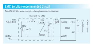
Note: 1.LD series meet the requirements of lightning protection. If the application requires higher performance for lightning protection and EMI, our standard products LH series (surge level three), LH-ER2 (surge level four) and recommended peripheral circuit are available;
