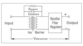
$$ILEAKAGE = \frac{V_{BREAKDOWN}}{R_{BARRIER}} = 2 \pi (60 \text{Hz}) (C_{BARRIER}) (240 \text{V})$$
