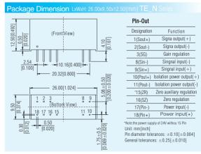
Active High Precision Output Signal Conditioning Module
