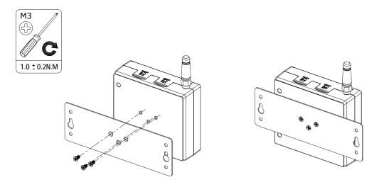
Use 3 pcs of ST2.9\*6 flat head self-tapping Phillips screws to fix the wall mounting kit to the gateway, and then use 2 pcs of M3 drywall screws to mount the gateway associated with the wall mounting kit on the wall.
