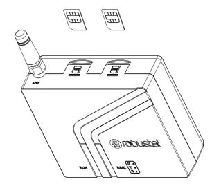
Please confirm before inserting the SIM card. When the SIM card is turned on and the device is configured without the correct PIN, the SIM card is unavailable.
