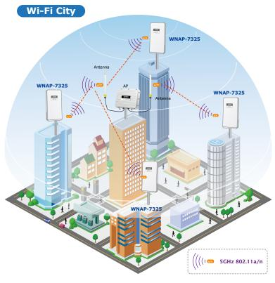
With built-in 14dBi dual-polarization directional antenna, the WNAP-7325 brings higher performance and longer distance of wireless connection. The WNAP-7325 provides high output power with multiply-adjustable Tx controller, which allows CPE users to easily install and adjust the suitable value in appropriate locations. Moreover, the WNAP-7325 supports WISP mode to enable CPE users to connect to Internet via local WISP provider.
