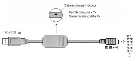
USB-SC09-FX programming cable simulate USB port as traditional serial port (usually COM3), which enables existing programming software(GX Developer) to communicate through simulated traditional port and PLC devices.
