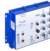
OCTOPUS OS32-080802T6T6TPEP (942 069-002) managed ruggedized IP65, IP67-Switch 10 TX, including 8 ports PoE (10/100 Mbit/s), M12 „D“ coding, 2x 1000 Mbit/s M12 „X“-coding Approvals: CE, C-Tick, GOST-R, EN 50155
