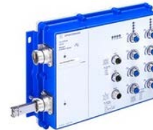
OCTOPUS OS32-0808020606TPEP (942 069-004) managed ruggedized IP65, IP67-Switch 10 Ports including 8 ports PoE, M12 „D“ coding, 2 ports 1000BASE-SFP sockets Approvals: CE, C-Tick, GOST-R, EN 50155
