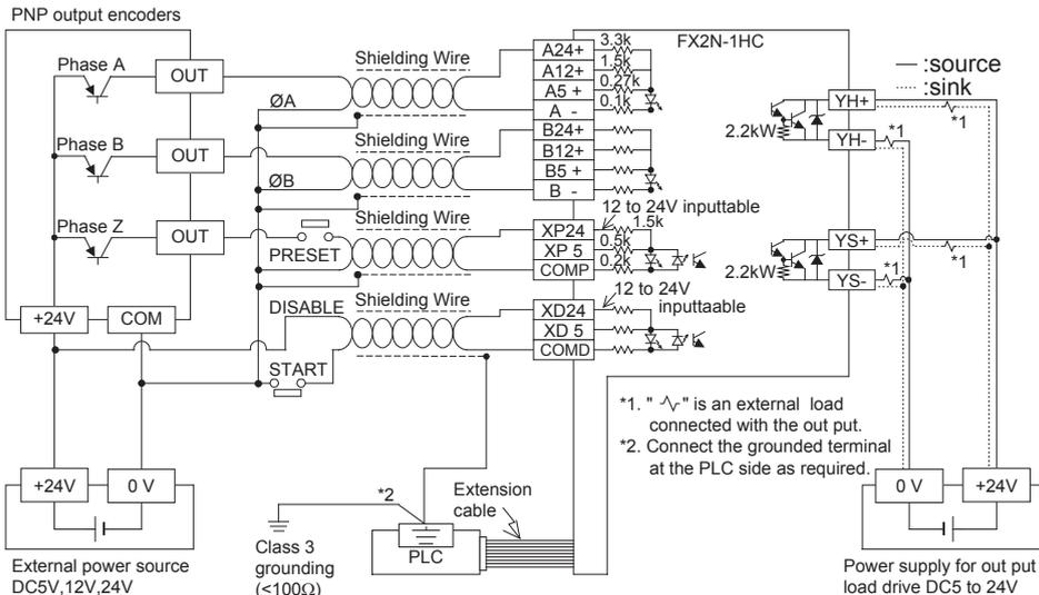
**!** If using on NPN output encoder please take care to match the polarity of the terminals of the encoder to those of the FX2N-1HC.
