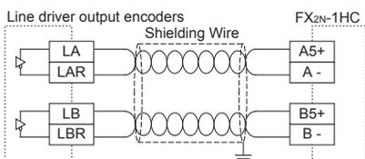
When applying the Differential-Line-Driver encoder (AM26C31 or equivalent) to FX2N-1HC, connect the encoder output with the 5V DC terminal as shown in the left figure.
