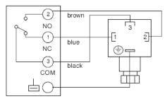
Fig.3. C6097A connection diagram with DIN plug
