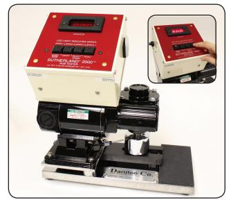
▲ Sutherland Rub Tester showing two pound and four pound weights and the scoring device. The upper receptacle of the timer is for remote timer control. The lower receptacle is the same voltage as the instrument. !
