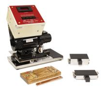
strokes. A single mounting pad for the test strip is cut to fit the weight. Two pound and four pound weights and scoring fixture are included.
