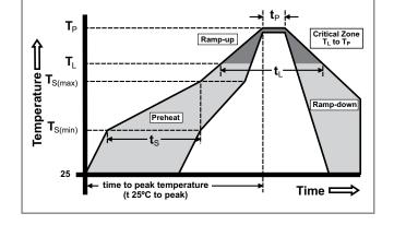
**Wave Soldering Parameters**
